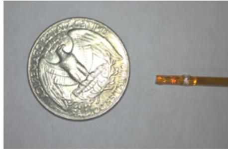
Fig. 3. Photo of qOCE probe in comparison with a US quarter.
