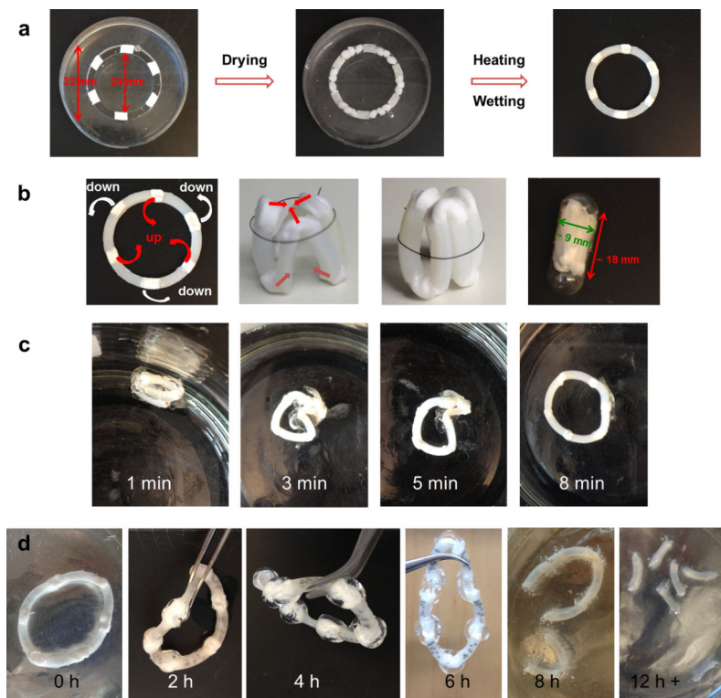
Figure 3. Construction of a ring-shaped gastric retentive device and in vitro testing of its elasticity and enteric property. a, Construction of a circle composed of polycaprolactone (PCL) arcs with intervening EE polymer gel linkers by first fitting cubic polymer gels and PCL beads alternatively in a circle-shaped polydimethylsiloxane (PDMS) mold followed by melting PCL at 70 °C. b, Folding of the ring into a standard gelatin 000 capsule by utilizing the elasticity of the polymer gel. c, Escape from the capsule and recovery to the ring shape after dissolution of the gelatin capsule in SGF at 37 °C. d, Progressive dissolution of EE supramolecular polymer gel linkers in SIF at 37 °C for the dissociation of the circle-shaped device into PCL arcs by utilizing the enteric property of the polymer gel.
