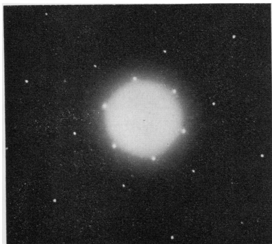
Fig. 5 A typical diffraction pattern obtained from single crystals in kidney or brain. The axial ratio is consistent with that of calcium oxalate dihydrate.
