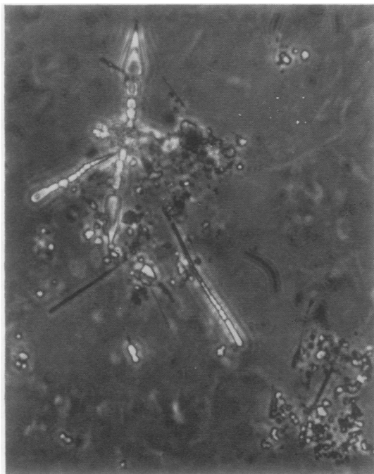
Fig. 2 The same field as in fig. 1 but under phase-contrast illumination. Several uncoated asbestos fibres are seen as well as coated ones. \times 400 .
