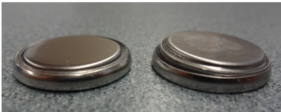
Figure 4. Coin cell that has been properly crimped (left) and improperly crimped (right). An improperly crimped cell will be noticeably open immediately after crimping or can pop over several hours later. Please click here to view a larger version of this figure.
