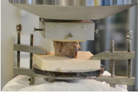
FIGURE 2: Experimental setup for mechanical testing. L2 vertebra is embedded with a two-component adhesive, placed in holding devices, fixed in hydraulic clamps, and loaded by a pressure plate on the upper vertebral body end plate.
