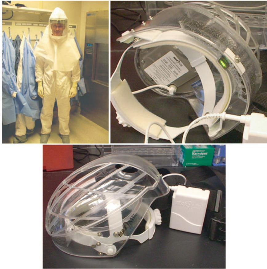
Fig. 14. The MaxAir PAPR System and the proper donning of this system. The shroud is placed over the helmet ( right side of figure ) and the battery pack is attached to the inside of the full body suit.
