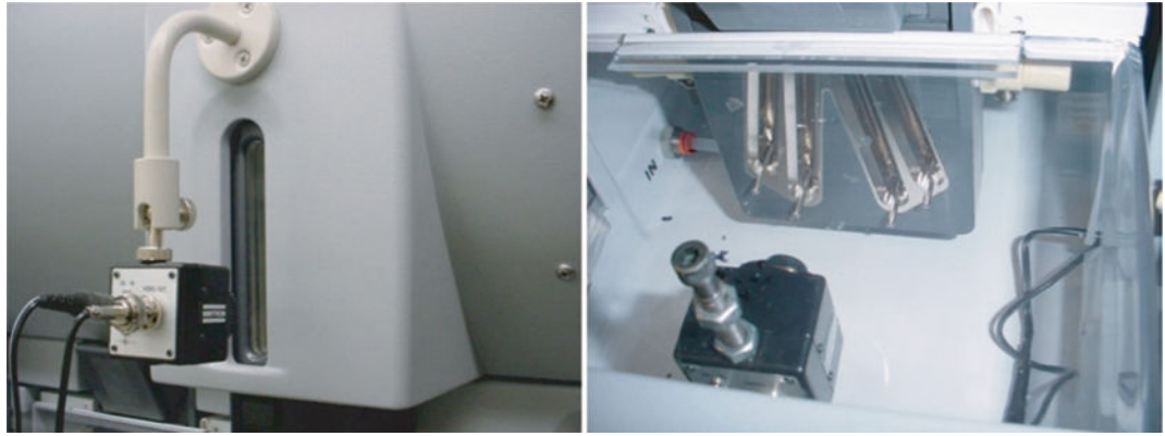
Fig. 2. Placement of cameras in front of the sample chamber and inside the collection chamber; output is sent to a video capture card in the acquisition computer.
