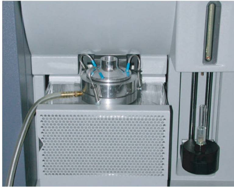
Fig. 8. Location of the collection area on an Aria I, which is directly outside on the closed sorting chamber.
