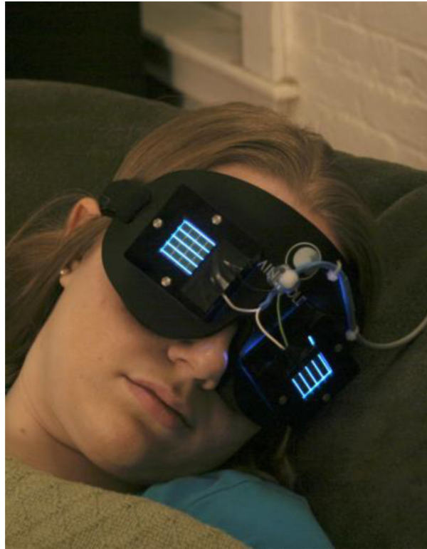
Figure 1. Active light was delivered through closed eyelids during sleep using a light mask. The light mask contained two blue LED arrays ( \lambda_{\text{max}} = 480 \text{ nm} , FWHM = 24 nm), one for each eyelid.
