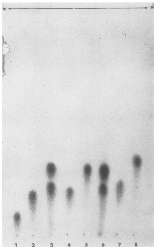
FIG. 4 Thin-layer chromatogram of sugars on a 20 \times 10 cm. plate (procedure as in text).
