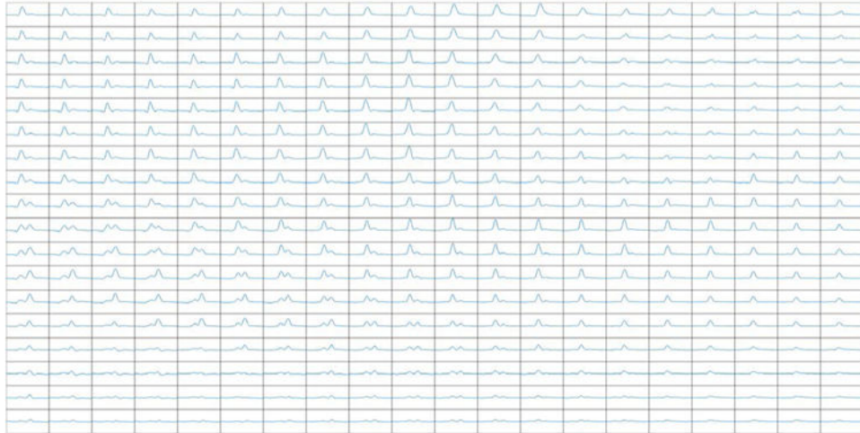
Array layout (18x20 channels) for a single detected spike from the Cat 1 data set
