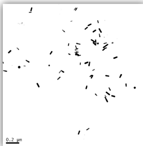
Figure 1. Transmission electron microscopy image of gold nanorods (GNRs).
