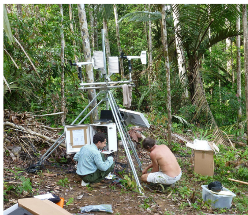
Fig. 4 Installation of an automatic weather station in the tropical rainforest in French Guiana (credits B. Hérault). Long-term monitoring of environmental conditions in remote forest inventory plots is a prerequisite to understand the effect of seasonal or extreme drought on tree and ecosystem functioning and simulate future changes
