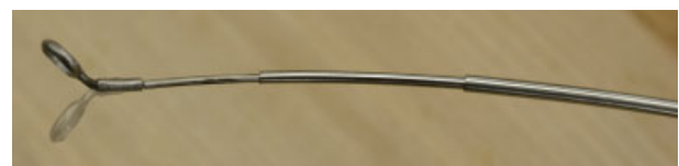
Fig. 3 The ability to rotate the ring curette axially while the robot arm remains stationary is illustrated in this image via a semitransparent overlay of a second configuration of the curette.
