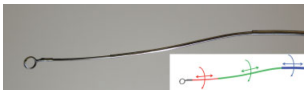
Fig. 1 A concentric tube continuum robot made from three precurved superelastic nitinol tubes. The robot is able to move like a tentacle by rotating and translating the tubes inside one another. Each of the 6 degrees of freedom is shown in the inset drawing. An angled ring curette, which can be axially rotated, is attached to the tip of the robot, similar to the curettes used in endonasal pituitary tumor removals.
