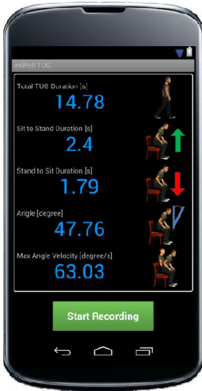
Fig. 4. Smartphone TUG application displaying the TUG parameters computed. Milosevic et al. (2013) [86].
