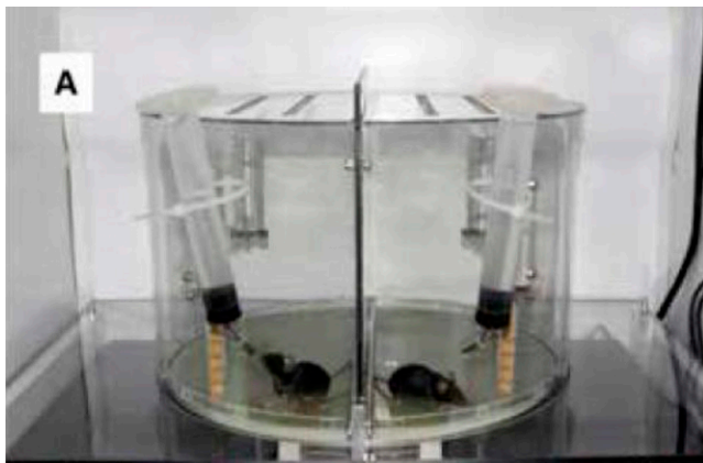
Figure 6. Sleep fragmentation device using a rotating disk. Reprinted with permission from Trammell and colleagues (60).
