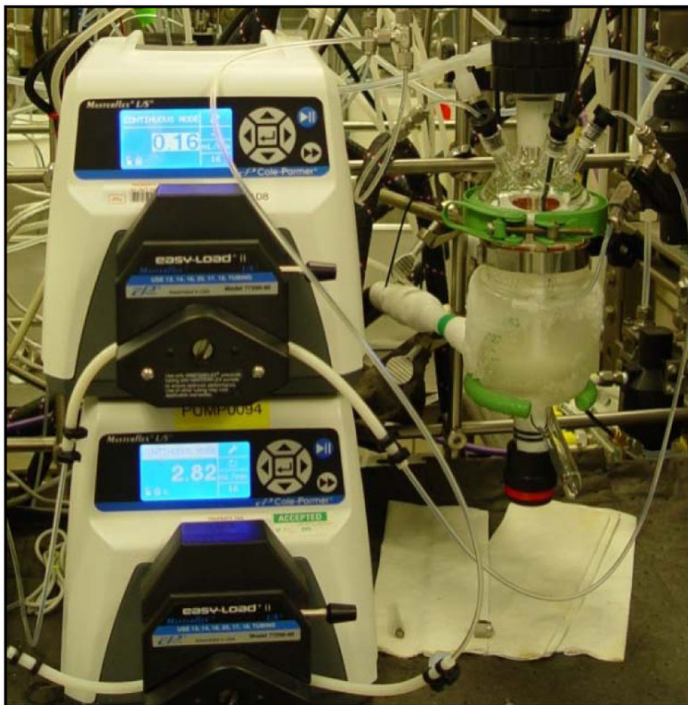
Figure 7. Reactor with a cooling jacket for the continuous crystallization process and peristaltic pumps used for the continuous feeding of solutions.
