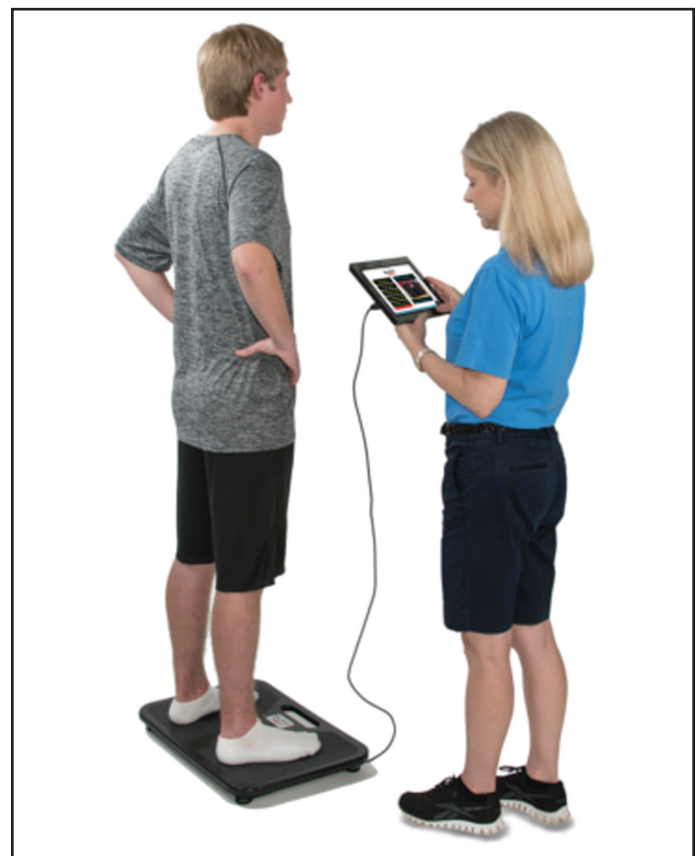
Figure 2. A depiction of the typical BBT administration. The athlete stands quietly on the BTrackS Balance Plate with eyes closed, feet shoulder width apart and hands on hips while the tester collects body sway information with a connected computing device running the BTrackS Sport Balance software.
