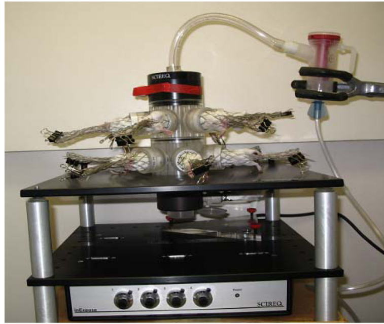
Figure 3. InExpose™ (SCIREQ®) nose-only exposure system.
