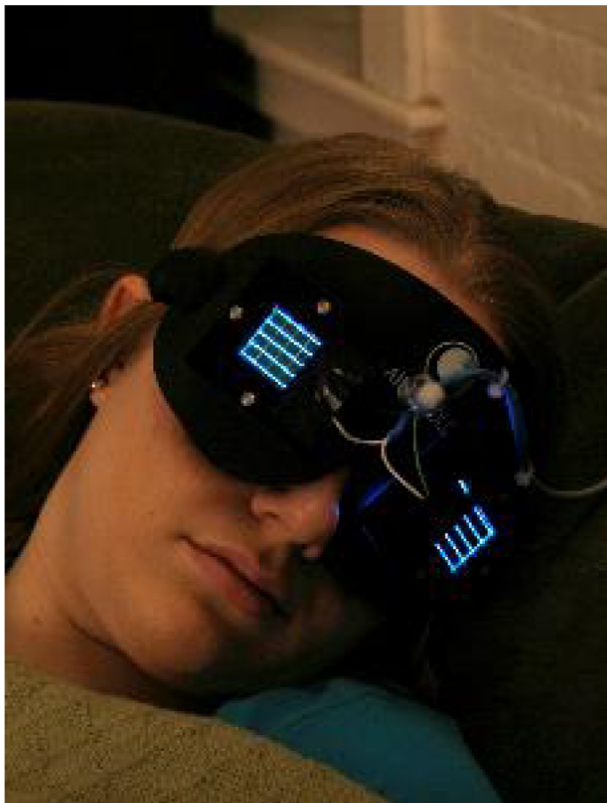
Figure 2 Flashing blue light mask used by older adults living at home. Notes: Flashing light was delivered through closed eyelids during sleep. The blue light mask shown here contains two blue LED arrays ( \lambda_{max} = 480 nm, FWHM = 24 nm), one for each eyelid. In the study, the light-stimulus condition was a train of blue or red light pulses: 2-second duration light pulses spaced apart 30 seconds, for no more than 3 hours, delivered before predicted minimum core body temperature. Photo courtesy of Lighting Research Center, Rensselaer Polytechnic Institute. 95 Abbreviations: LED, light emitting diode; FWHM, full width at half maximum.
