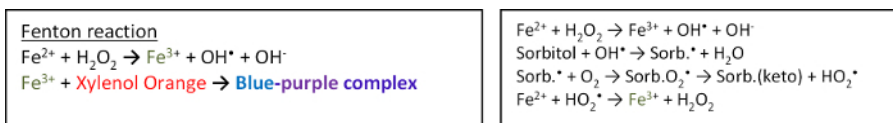
Figure 4. The FOX Method. White-rot fungi attack the cell wall of wood through a Fenton reaction that produces hydroxyl radical \text{OH}^{\bullet} . The FOX method couples this reaction to xylenol orange (XO), and the absorbance of the \text{XO-Fe}^{3+} complex is measured at 560 nm. Ferrous oxidation is amplified by the addition of sorbitol to the reagent mixture. Please click here to view a larger version of this figure.
