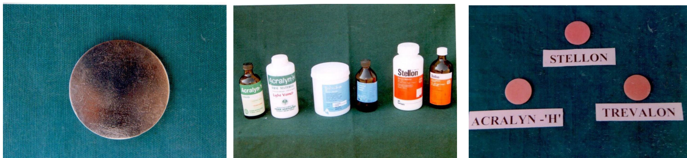
[Table/Fig-1]: Circular metal disc used to prepare acrylic specimens. [Table/Fig-2]: Resins used in this study. [Table/Fig-3]: Resin specimens of three different brands.
