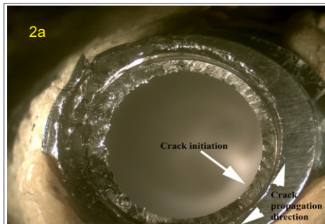
Figure 2a: Photograph of the fracture initiation site and direction of propagation around the taper junction.
