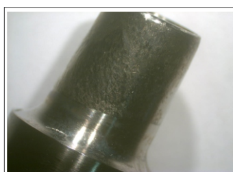
Figure 4: Photograph presenting mechanical fretting of the male taper junction.
