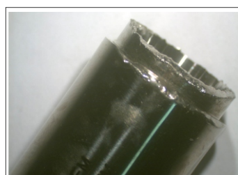
Figure 3: Photograph showing no fretting corrosion at the outer region of tibial taper junction.
