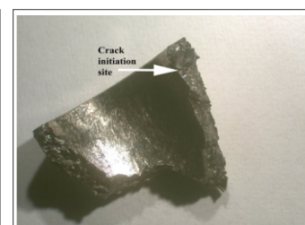
Figure 6: Photograph of a female taper junction fracture fragment showing a crack initiation site.
