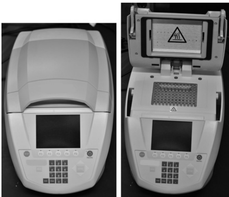
Figure 5. Thermal cycler. Closed thermal cycler left image. Right image contains 0.2 ml thin walled PCR tubes placed in the heating block of an open thermal cycler.
