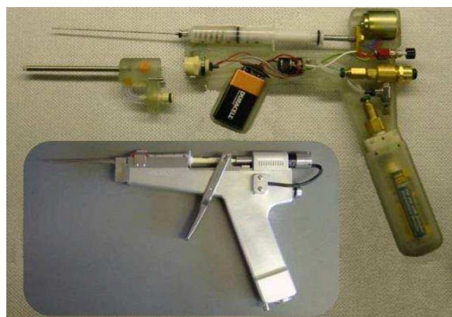
FIGURE 2. Student prototype ACL Repair Gun with inset showing second generation prototype.
