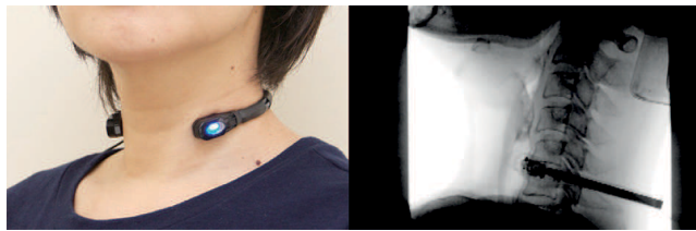
FIGURE 3. Microphone placement at the C5 level. Mild pressure from the spring characteristics of the neckband creates good contact between the skin and the microphone. The VF image shows a lateral view.
