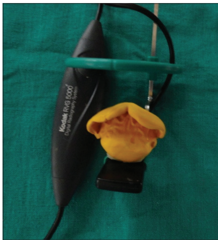
Figure 1: RVG sensor with Rinn XCP sensor holder with addition silicone impression
