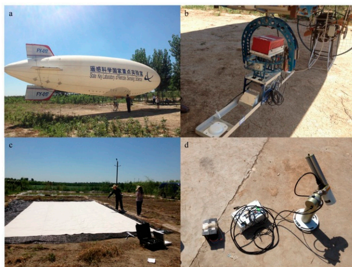
Figure 2. Experimental setup. (a) airship; (b) AisaEAGLE airborne Hyperspectral Imaging System; (c) reference white board; (d) CE318.
