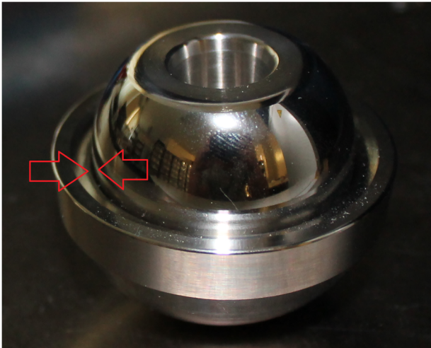
Figure 2 A Pinnacle head and liner. The red arrows indicate the small gap between the head and the liner surface which is the 'clearance'. Diametrical clearance is calculated by subtracting the diameter of the head from the diameter of the liner.
