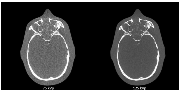
FIG. 7. CT images of the anthropomorphic head phantom. The white box on the 75 kVp image outlines the insert region shown in Fig. 9. Display window: [-500\ 1000] HU.
