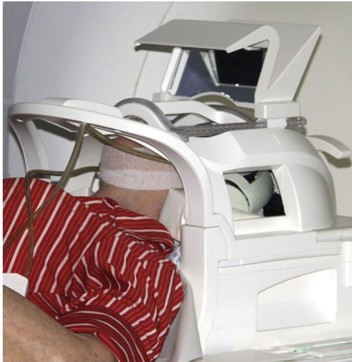
Fig. 10 – Extra oral head and neck coil. Positioning of the patient with a 20 channel head and neck coil inside the Siemens Skyra 3.0 T MRI. (Reprinted, with permission from Elsevier, Assaf et al., Evaluation of four different optimized magnetic-resonance-imaging sequences for visualization of dental and maxillo-mandibular structures at 3 T. J Craniomaxillofac Surg 2014;42:1356–63).
