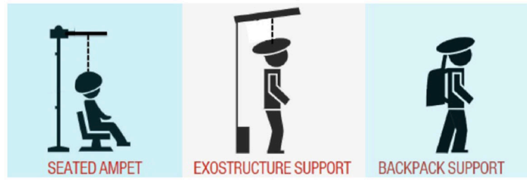
Figure 1. The three proposed working designs for the ambulatory micro-dose brain PET imager (AMPET).
