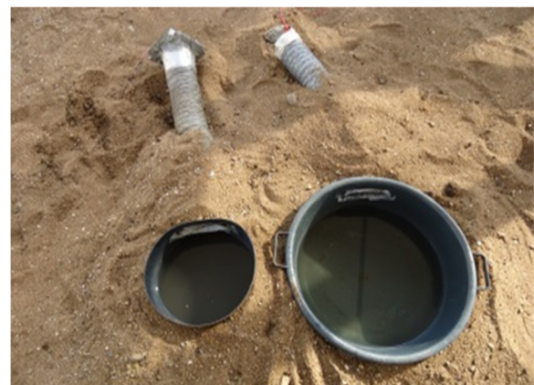
Fig. 3 Comparison of the prototype OviART gravid trap with small basin (left) and improved trap with a basin twice the size of the prototype (right)
