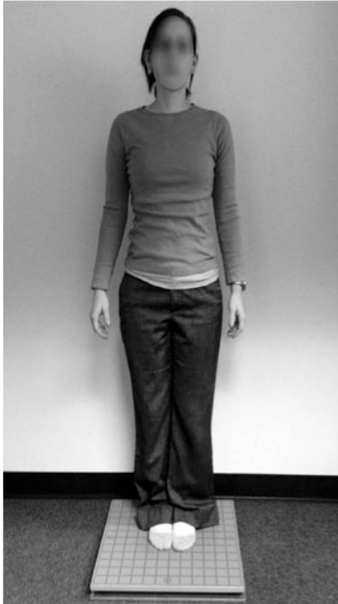
Fig. 2. This figure demonstrates an example of the administration of a force platform protocol to measure center-of-pressure (COP) trajectories.
