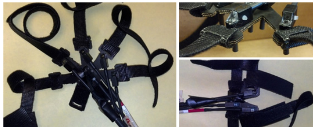
Fig. 2. Head probe arrays for the DLPFC (left) and the MFG (lower right). Prisms and light pipe assemblies (top right) were used with optical fibers.
