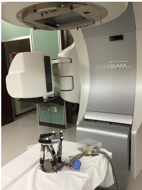
FIG. 3. Experimental setup for the test of the calibration methodology using an IR marker tracking system. Shown are the robotic motion phantom with a set of four reflective IR markers fixed to the top platform, which were tracked using the stereoscopic IR camera (not shown). The arrangement of the four markers produces a virtual point for tracking, which is called the M frame of reference.
