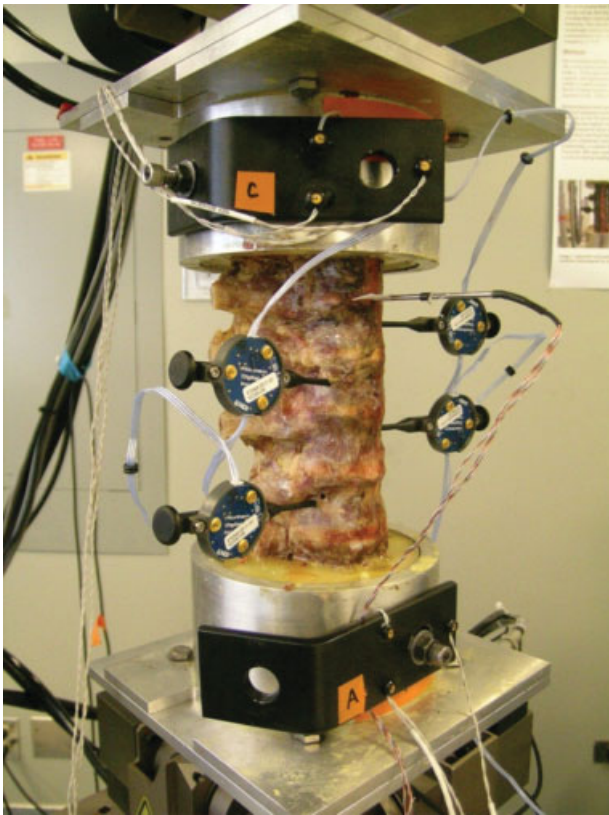
Fig. 1 Specimen mounted on MTS testing machine (MTS Bionix 370.02, MTS Systems Corp., Eden Prairie, Minnesota, United States), equipped with “spine pin” infrared rigid body markers and intervertebral disk pressure sensor needle.
