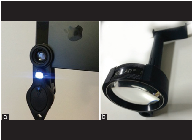
Figure 1: The EyeGo system including (a) an anterior adapter consisting of a macro lens and LED light and (b) a three-dimensional printed posterior adapter to help align a 20D lens with the phone's camera
