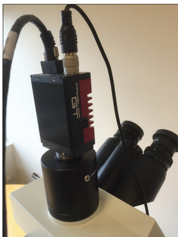
Figure 1: Prosilica GT camera attached via a C-mount to a microscope was used to manually acquire panoramic digital images
