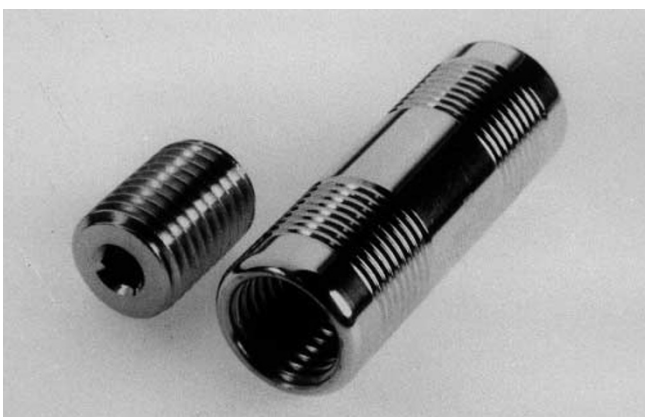
Fig. 1 The modified keyed centering sleeve with the custom bolt
