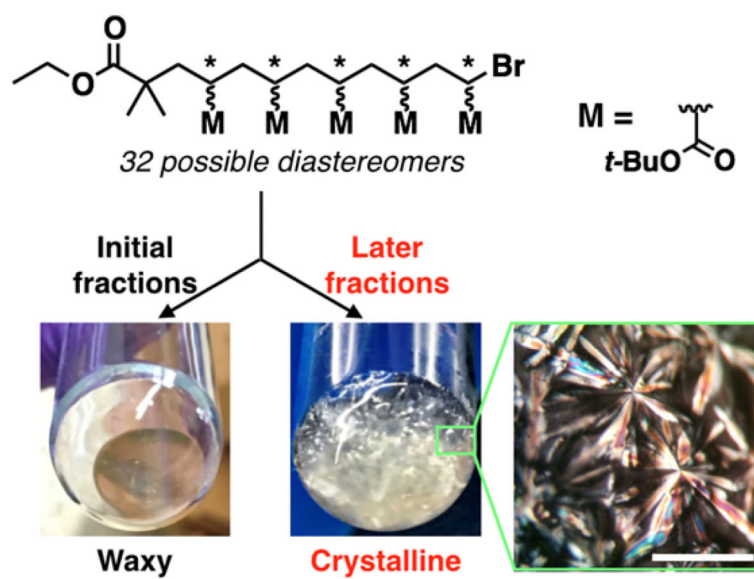
Figure 4. Variation in physical appearance for n = 5 penta-TBA 5 derivatives. Initial fractions were obtained as a waxy solid with later fractions being crystalline. Inset: polarized micrograph of crystalline penta-TBA 5 , scale bar is 1 mm.
