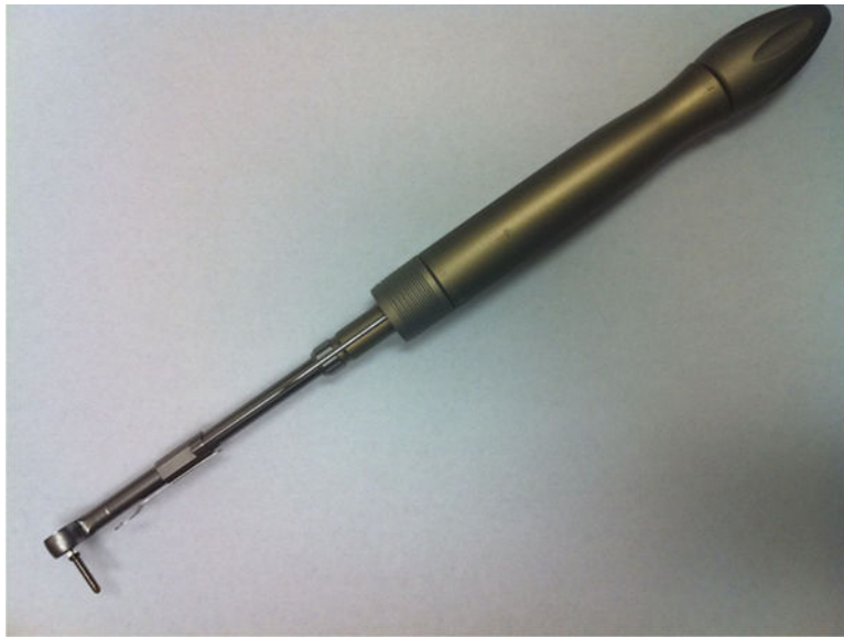
Fig. 3. A 90° drill and screwdriver
