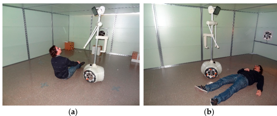
Figure 18. Simulation of the APR used as a fall detector (a) with activity and (b) without activity.
