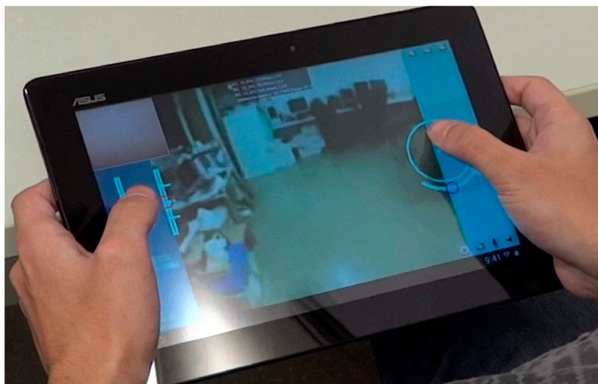
Figure 7. Android APP used for the remote control of the APR.
