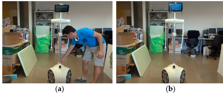
Figure 12. (a) Starting the APR; (b) APR initializing the onboard sensors and initializing the Tablet of the head.
