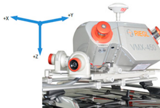
Figure 1. The coordinate system of the RIEGL VMX-250. Axis X, vehicle travel direction; Y, vertical on top of rails and pointing up; Z, perpendicular to the XY plan in the nadir direction.
