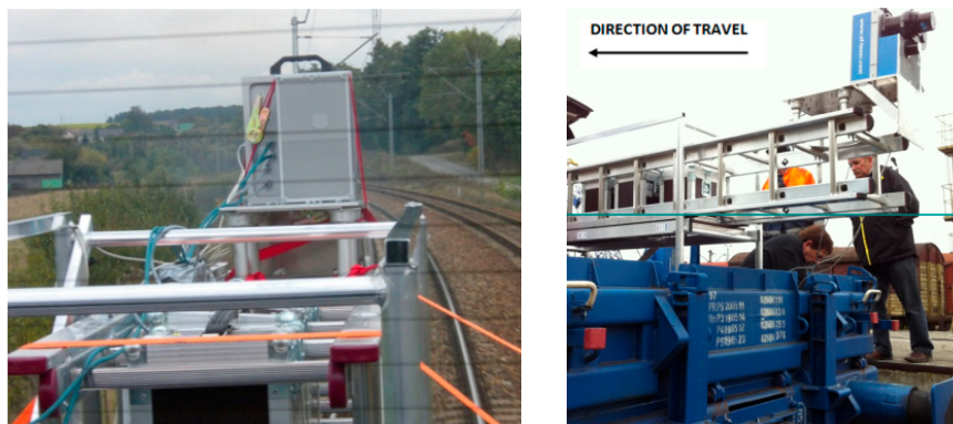
Figure 4. System 1: Z+F Profiler 9000 scanner on a railroad carriage. In the picture, the installation of the Z+F scanner and construction on the platform are shown ((left) rear view; (right) side view).
