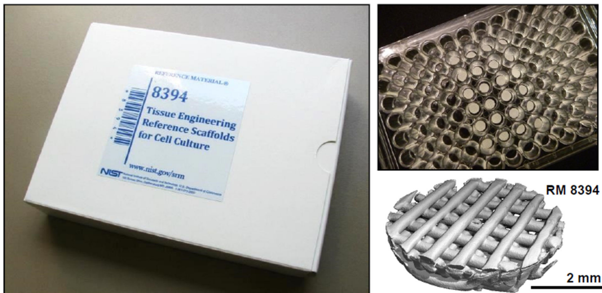
Fig. 2. NIST reference material scaffolds. (a) RM8395, RM8396 and RM8397 are freeform fabricated scaffolds with 3 different strut spacings, 200 \mu\text{m} , 300 \mu\text{m} and 450 \mu\text{m} , respectively. They are characterized for structure and porosity. (b) RM8394 is a set of 24 freeform fabricated scaffolds in a 96-well plate and are characterized for cell adhesion and proliferation.
