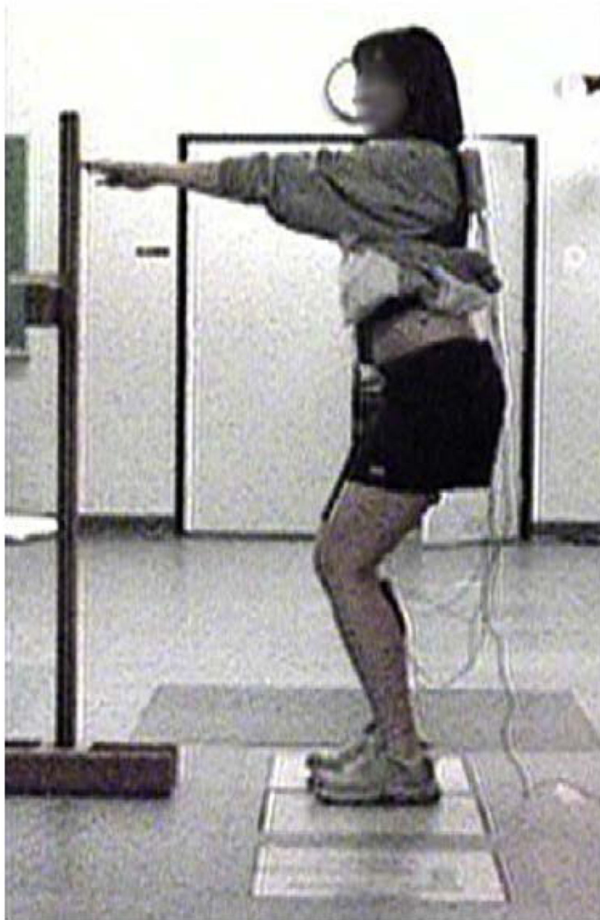
Fig. 1. The experimental set up for the squat maneuver used to estimate quadriceps muscle forces.
