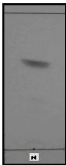
FIGURE 1: TLC profile of the active fraction [developing system: n -hexane : ethyl acetate (4 : 1), visualisation: UV -254 nm].
