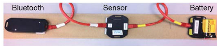
Figure 1. The National Institutes of Health Toolbox device. The sensor (middle) is shown along with its power supply (right) and Bluetooth wireless device (left).
