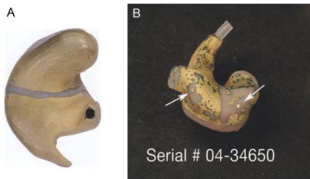
Figure A1 Photographs of first-generation sound generators/placebo sound generator shells. (A) Unworn device prior to participant use. (B) Worn device at end of treatment when placebo device failure was determined by General Hearing Instruments (GHI, Harahan, LA) for the participant assigned to group 2 but moved to as-treated group 1. Note the significant erosion of the gold plating from the surface of the failed worn device, which precluded normal placebo function.
