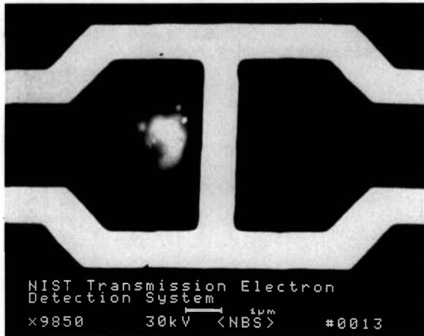
Fig. 30. TED mode as applied to x-ray mask repair. (a) Micrograph with intentionally ion-beam-milled windows positioned 1 micrometer from the edge using the Micron ion beam mask repair system. (b) Defect in the absorber to be repaired.
