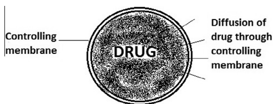
Figure 5 Mechanism of drug release through polymer matrix.
